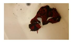
Fire in residence hall. A scarf was placed over a lamp shade creating enough heat to melt shade and catch scarf on fire.
